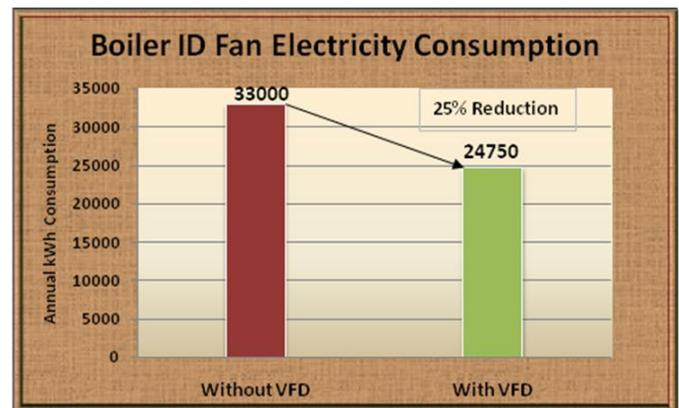
**By installation of VFD on ID Fan of Boiler reduces 25% of Electrical Energy consumption**
